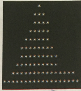
FIGURE 2 – Display of an histogram; abscissa : pixel value k ; ordinate : n_k ; in this example, only a subset of the histogram is shown.
