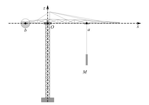
The liquid can be pumped into the sphere to fill it up (making it heavier) and out of the sphere (making it lighter), to adjust the counterweight. The mass of the empty spherical tank is considered as negligible.
