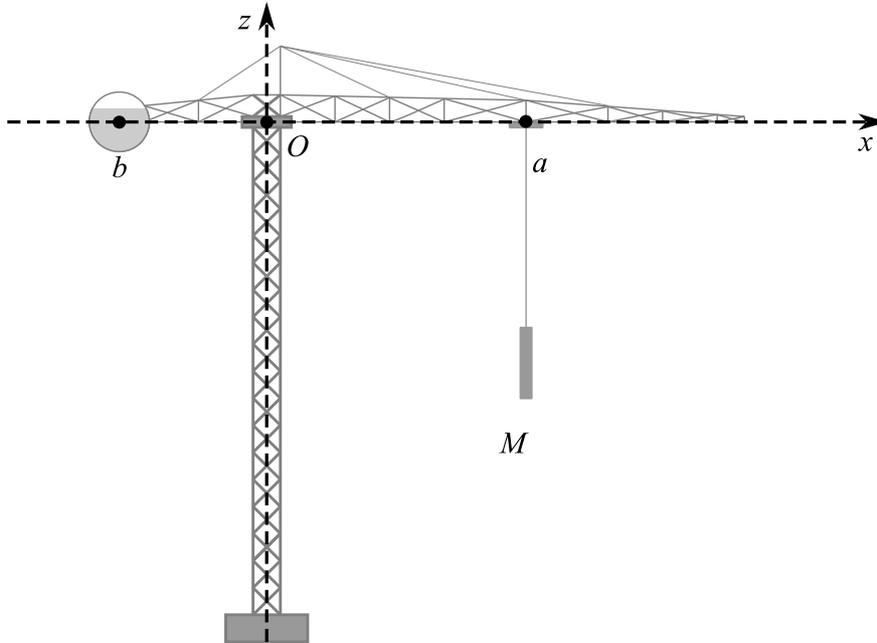
The liquid can be pumped into the sphere to fill it up (making it heavier) and out of the sphere (making it lighter), to adjust the counterweight. The mass of the empty spherical tank is considered as negligible.
