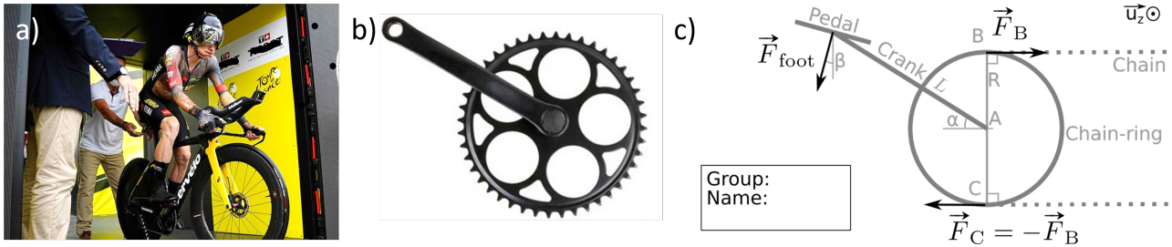
Figure 2: a) Picture of a cyclist at the start of a time trial. b) Picture of a bicycle drive (“pédalier” in French). c) Scheme of the bicycle drive. Some of the forces are represented.
