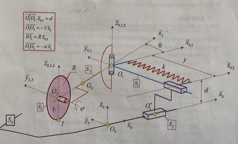
Figure 1: Scheme of the lower part of the landing gear.
