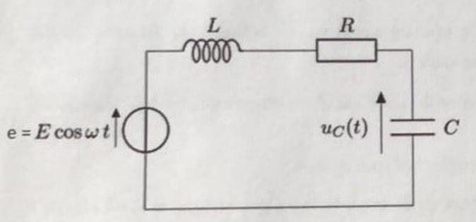
We consider the circuit represented in figure 1 with R=10  $\Omega$ , L=100 mH and C=10  $\mu$ F.
